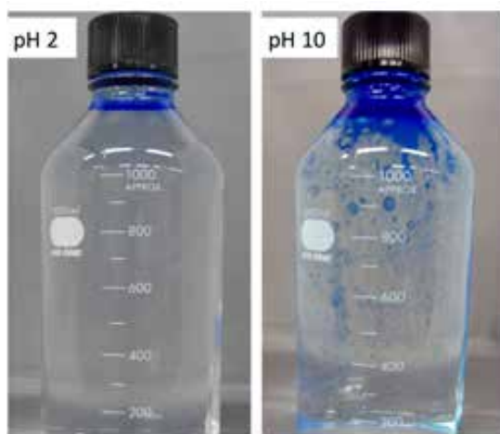
Fig. 2 pH-responsive oleophobicity of our polymer brush surface: This superoleophobicity can be activated (left image, pH = 2) and deactivated (right image, pH = 10) by changing the solution pH. Reprinted from ACS Appl. Mater. Interfaces, 2014, 6 (15), Dunderdale et al Large-Scale and Environmentally Friendly Synthesis of pH-Responsive Oil-Repellent Polymer Brush Surfaces under Ambient Conditions, 11864-11868, © 2014, with permission from ACS.
